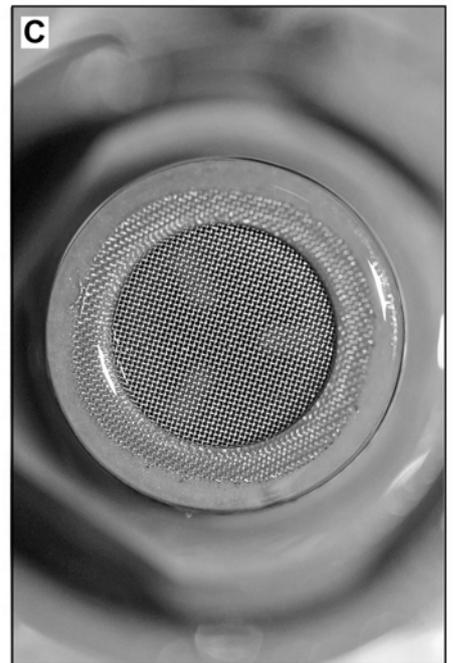
**A** If the control solenoid valve looks like this after cleaning, it needs to be replaced
