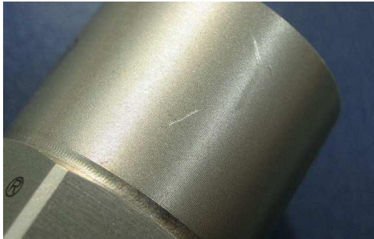
Figure 12 Unacceptable Scratches on Part Example
